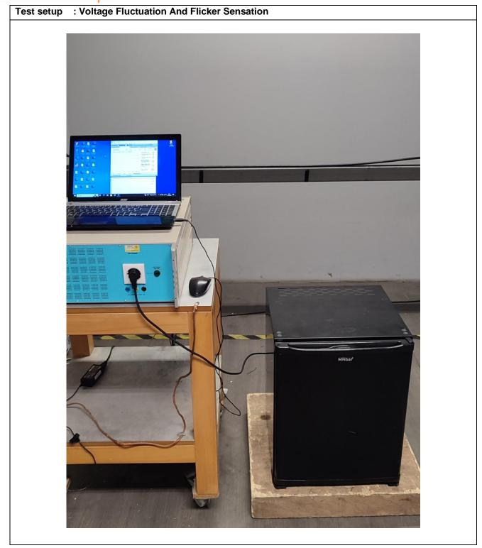
**TEST SUMMARY P** The EUT fulfill the requirements of the EN 61000-3-3.
