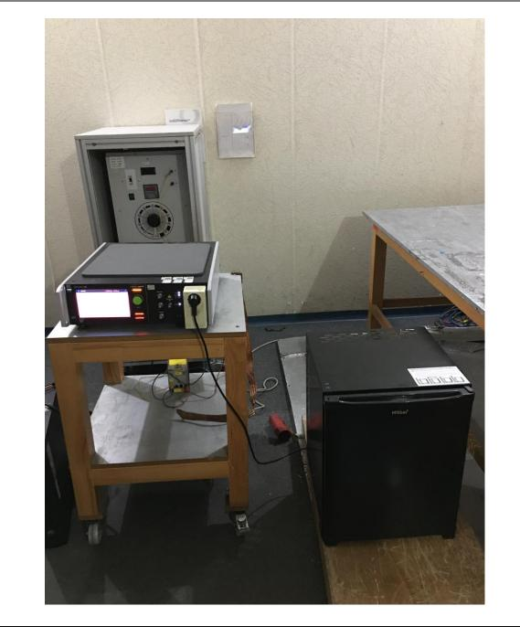
TEST SUMMARYPThe EUT fulfills the requirements of the EN 61000-4-5 with Criteria B.
