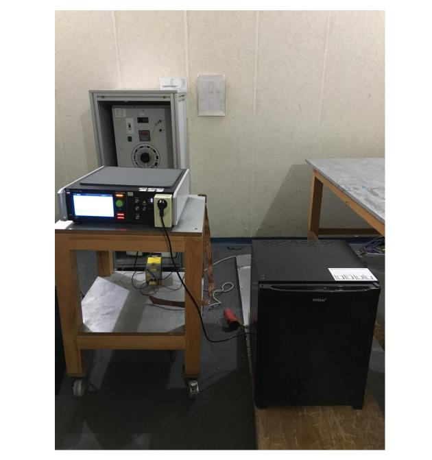
**TEST SUMMARY P** The EUT fulfills the requirements of the EN 61000-4-4 with Criteria B.
