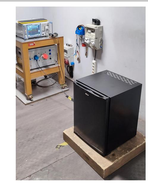
**TEST SUMMARY P** The EUT fulfills the requirements of the EN IEC 55014-1 Conducted Emission part.
